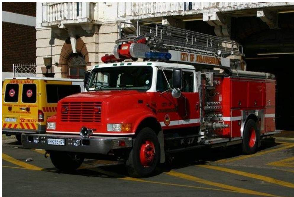
E-One Telesquirt "Boom Pumper", classed as First Turn Out but has better ladder capability's
