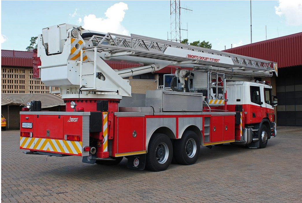
Bronto Aerial Platform Vehicle City's Tallest Aerial Appliance
